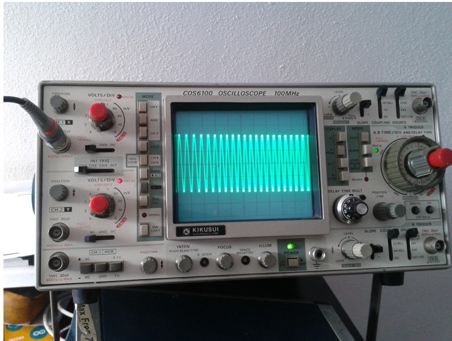
Figure 5: Clock Oscillator test with an Oscilloscope.
