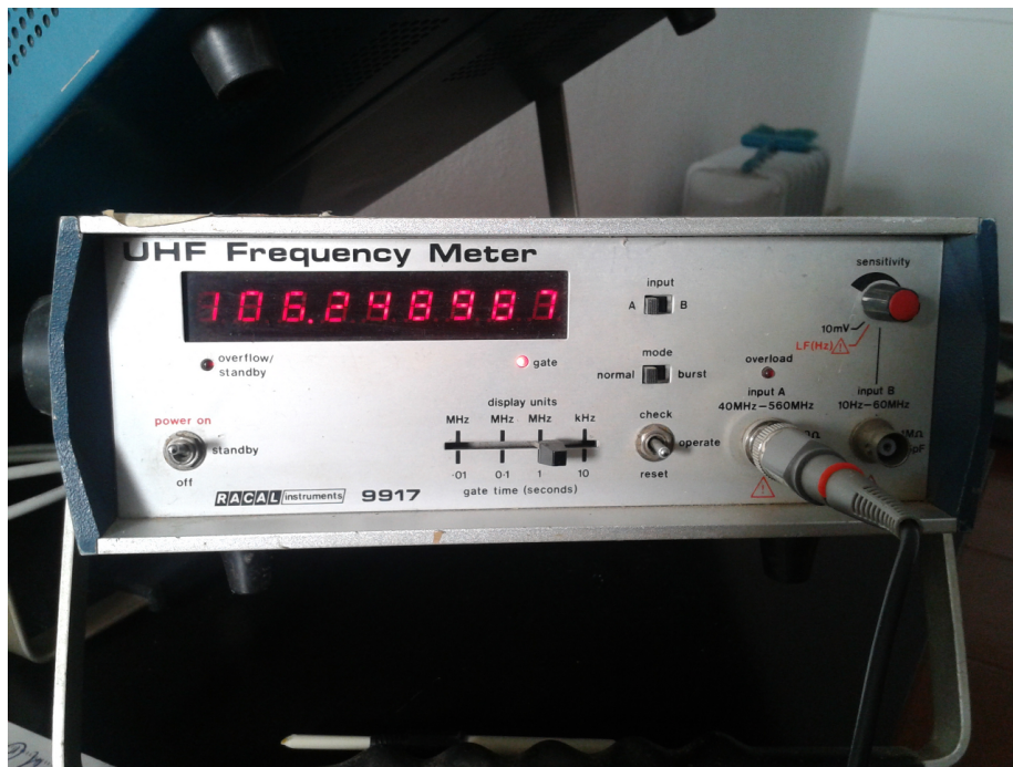
Figure 6: Clock Oscillator test with a Frequency Meter.
